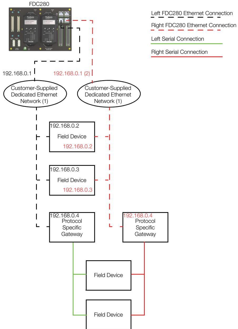
(1) When connecting to field devices via a network, we recommend using managed switches for maintenance and troubleshooting. Network is optional.
