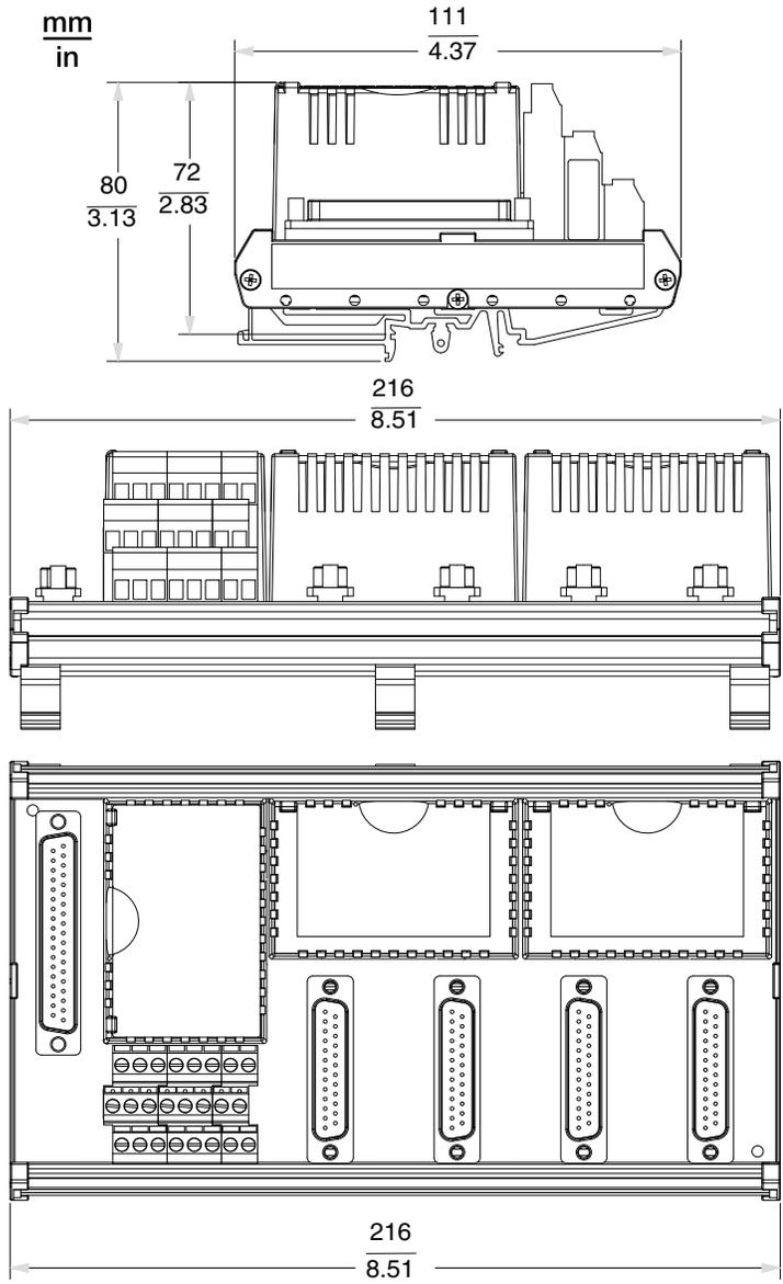
Figure 11 - Ring Lug Termination Assembly (P0926PA)<sup>(1)</sup>
