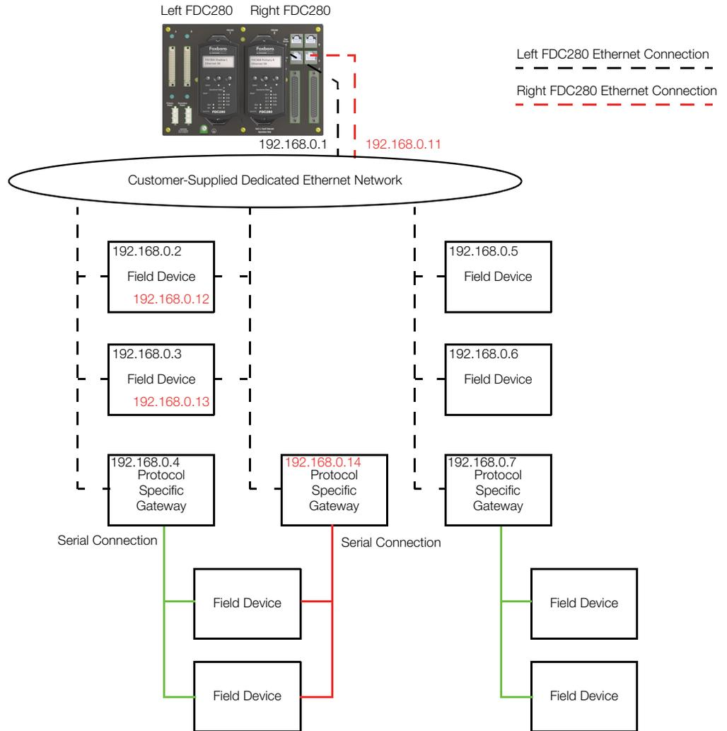
(1) We recommend using managed switches for maintenance and troubleshooting. However, field devices may also connect directly to the FDC280 baseplate without the Ethernet switches or hubs, which are part of the customer-supplied Ethernet network.
